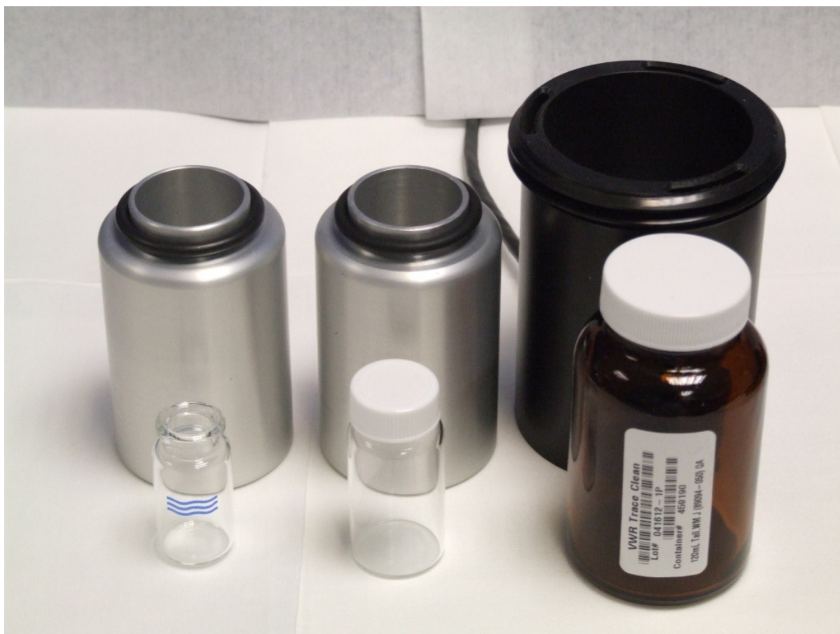
Figure 3 The vials, inserts and bottles available for use in the ATLAS Sampling Module
