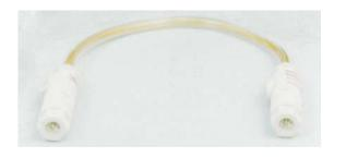
This one-of-a-kind membrane dryer is used in low air flow applications where space is at a premium. The dryer can be bent to go through tight spaces between other components. The flow pattern is bi-directional, the inlet can be either of the 1/4" end ports.
