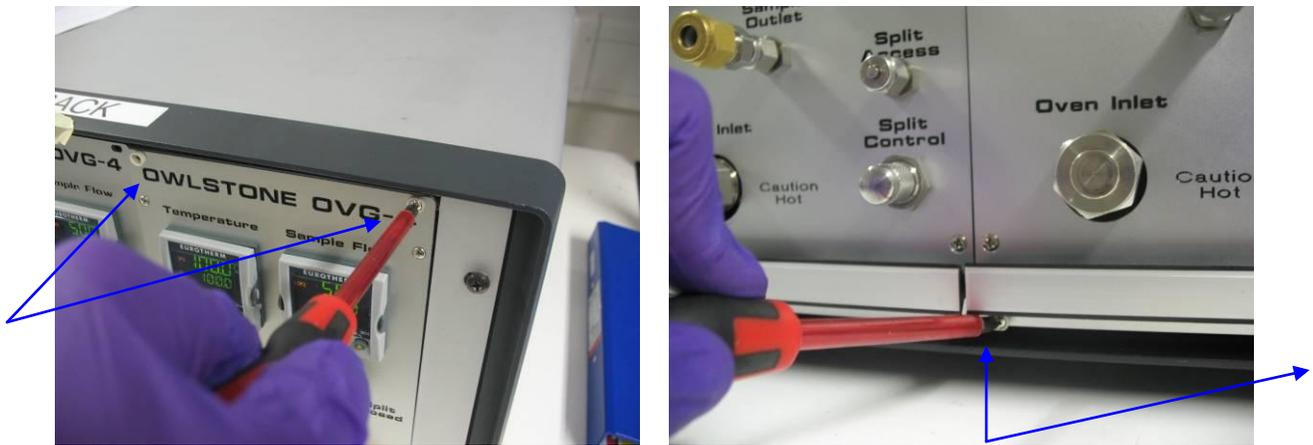
Figure 7 – photograph showing the 4x screws used to mount the OVG-4
