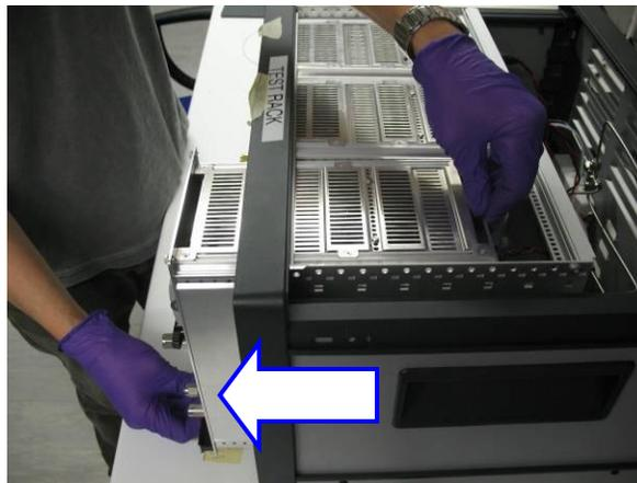
*Figure 12 – removing an OVG-4 from the GEN-SYS rack*
