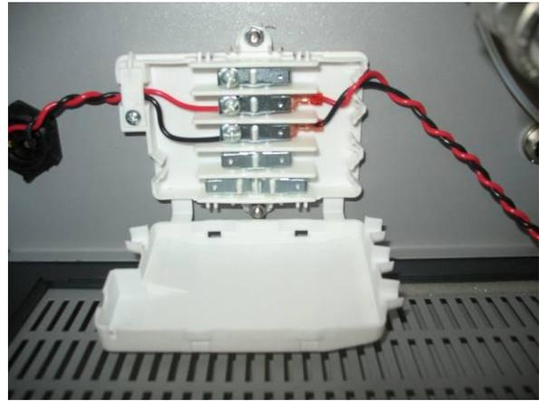
Figure 21 – terminal box with 1x DC power cable
