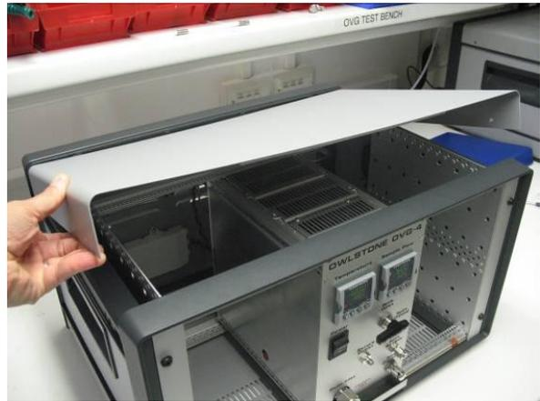
Figure 8 - removing the roof panel
