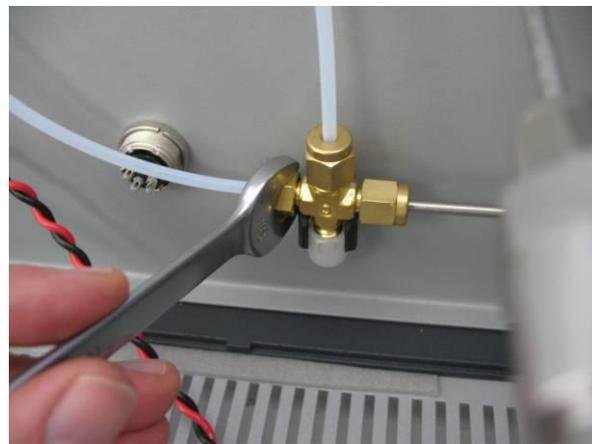
Figure 19 – installing the new exhaust lines
