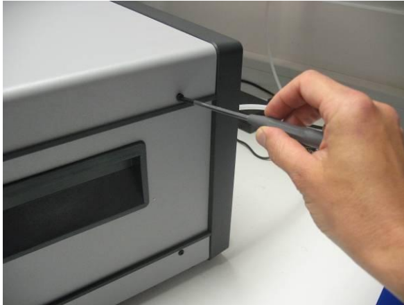
Figure 5: removing the roof panel
