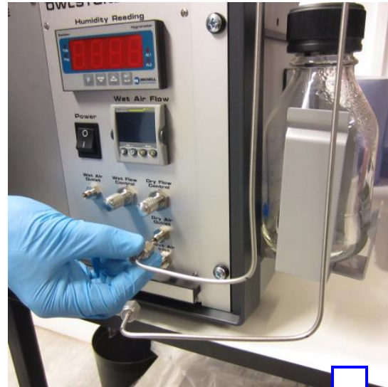
Figure 25: attaching the pipes
