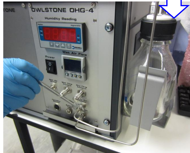
Figure 26: attaching the pipes
