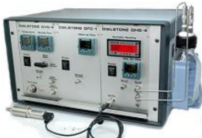
**The Owlstone Vapour Generator (OGV-4) is a compact, cost effective calibration gas system, which can generate NIST traceable, precise, repeatable and accurate concentrations of chemicals and calibration gas standards.**
