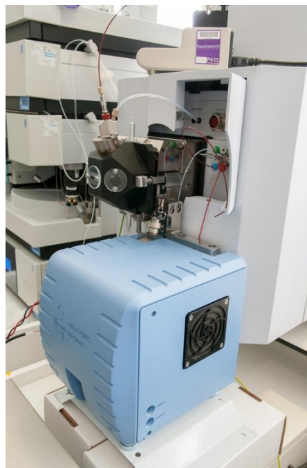
UltraFAIMS-B1 mounted on Bruker Impact HD with Apollo II electro spray source
