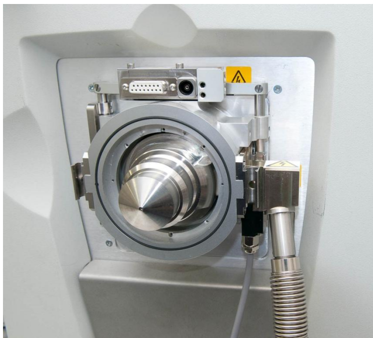
UltraFAIMS-T1 mounted on Thermo Exactive with Advion Nanomate source
