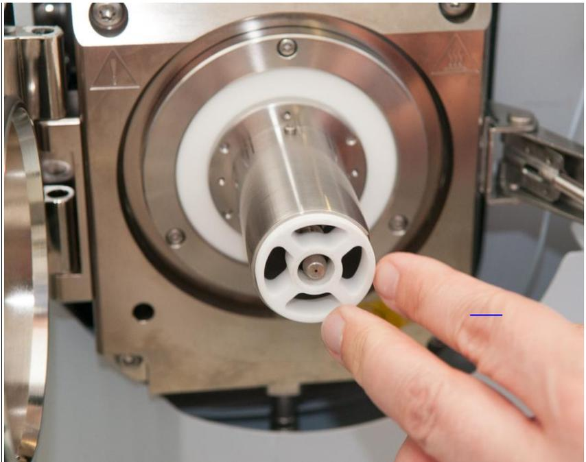
13. Swing the adaptor back into the closed position, then push the chip holder (the loose end of the waveform feeder) into position on the capillary extender.
