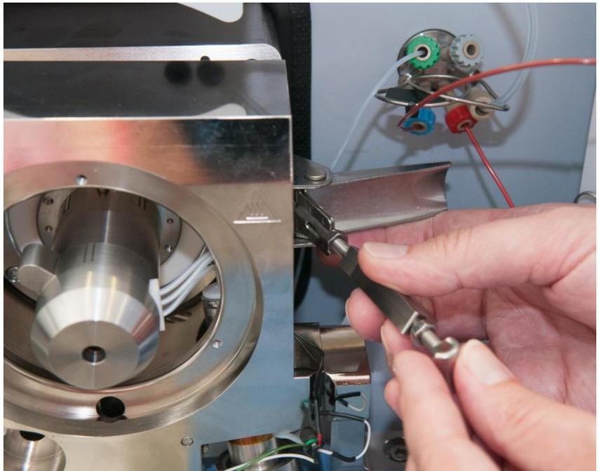
17. Mount the separation disk, if required, using the small screws provided.
