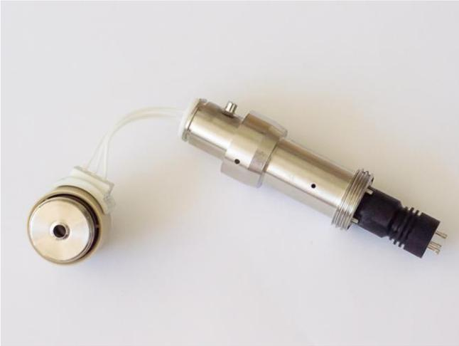
The waveform feeder connects the chip to the control unit so that the FAIMS waveforms can be applied.
