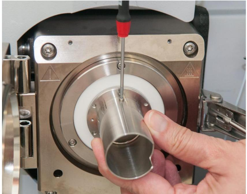
11. Push the capillary extender onto the capillary.
