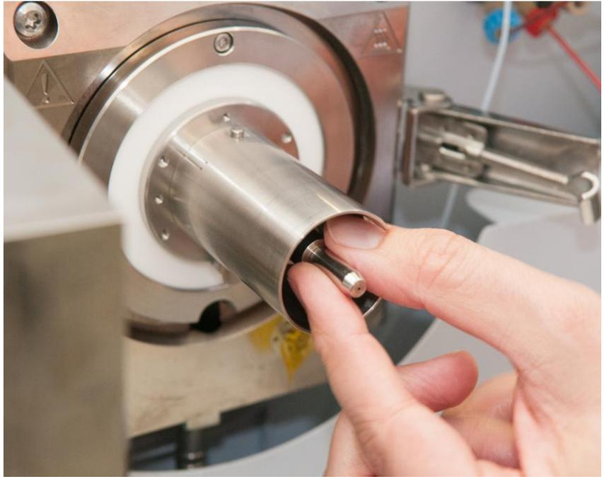
12. Fit the capillary support over the capillary extender and push it into place (until it hits the stop)
