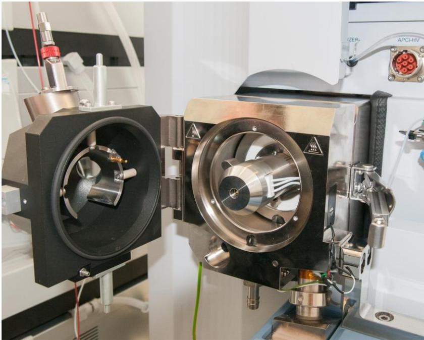
2. When cool enough to handle, slide the spray shield off.
