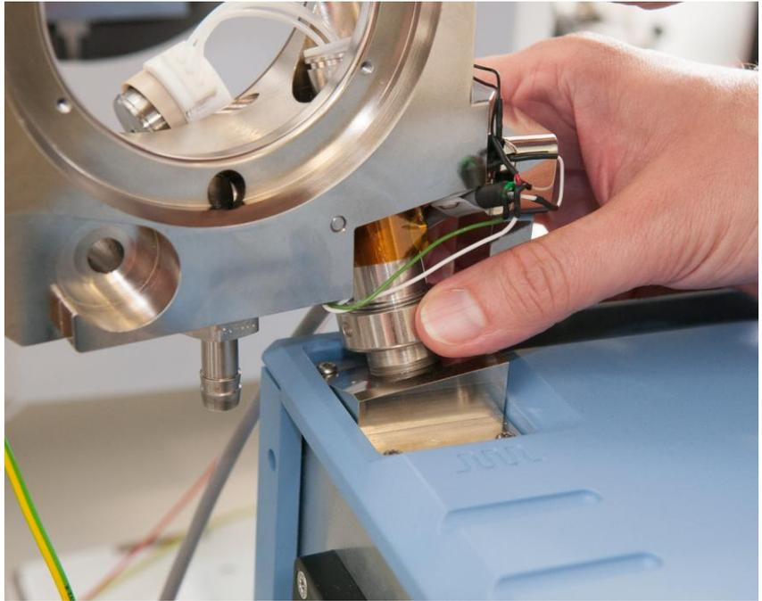
7. Fit the remaining two screws in the attachment bracket to secure the adaptor at the correct height.
