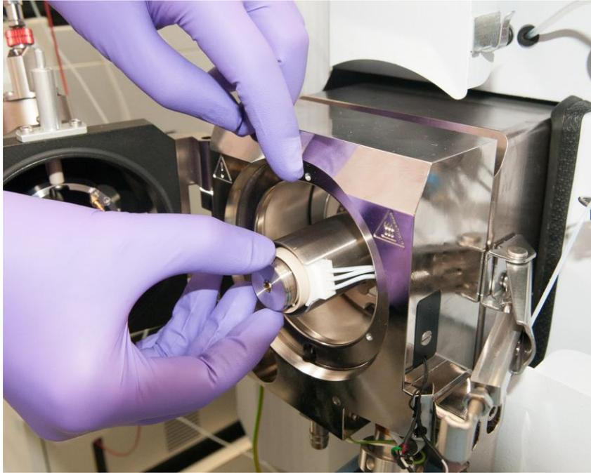
4. The chip module can be cleaned by immersing in suitable solvents and sonicated, or by heating (up to 150°C). Exposure to vacuum (e.g. in vacuum oven) is not recommended and may distort the chip mount. Ensure the chip is completely dry before applying FAIMS waveforms to the cleaned chip. Further advice on cleaning can be found on the Owlstone support website (<http://support.owlstonenanotech.com/categories/20097286-UltraFAIMS>)
