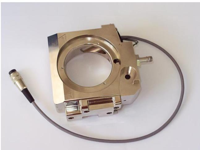
The adaptor assembly is the interface between the mass spectrometer, the FAIMS module and the ionisation source.
