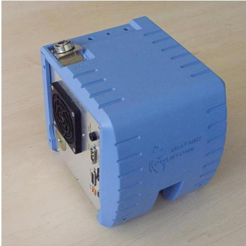
The control unit generates the FAIMS waveforms needed to drive the FAIMS chip. It is controlled by the PC software supplied.
