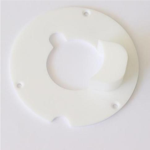
The separation disk can be used to block off the extra volume added to the source chamber by the adaptor assembly, in order to keep gas flow patterns within the ionization source as close as possible to the standard configuration.
