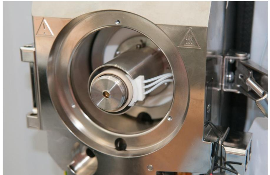
Note – when reversing these steps to uninstall the system, use caution when sliding the chip holder off the capillary extender. The capillary extender will initially slide forwards with the chip holder. Once the capillary support disk is visible, hold this in place to stop the capillary extender sliding further forward while you pull the chip holder off the capillary extender. **DO NOT STRETCH THE WIRES BETWEEN THE CHIP HOLDER AND THE WAVEFORM FEEDER.**
