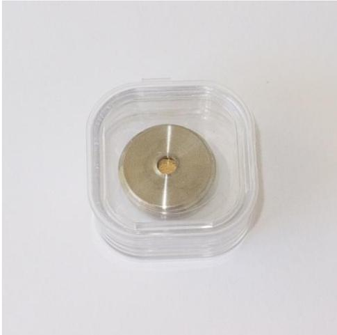
The chip is the core of the ultraFAIMS system – this is the FAIMS device that produces the separation of ions as they pass through the fields applied across the channel.
