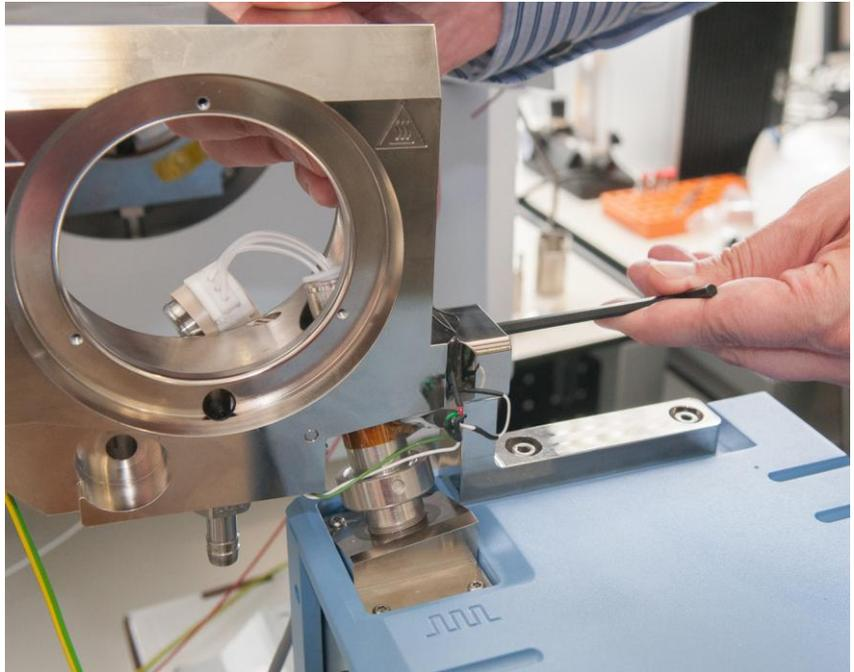
8. Lift or slide the adaptor plus control unit assembly into place, so that the adaptor block hinges line up with the hinges on the MS desolvation chamber. Secure the hinges with the locking pin provided.
