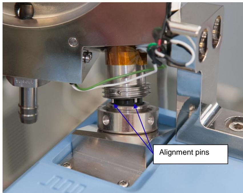
6. Tighten the locking nut to secure the waveform feeder in place.
