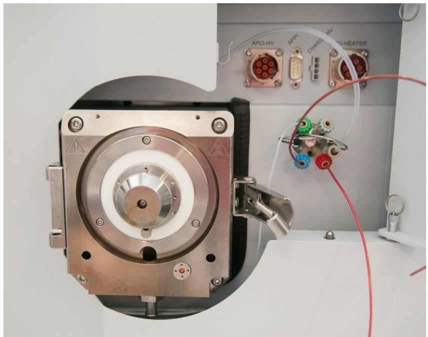
2. Remove the spray shield and capillary cap, leaving the bare capillary visible
