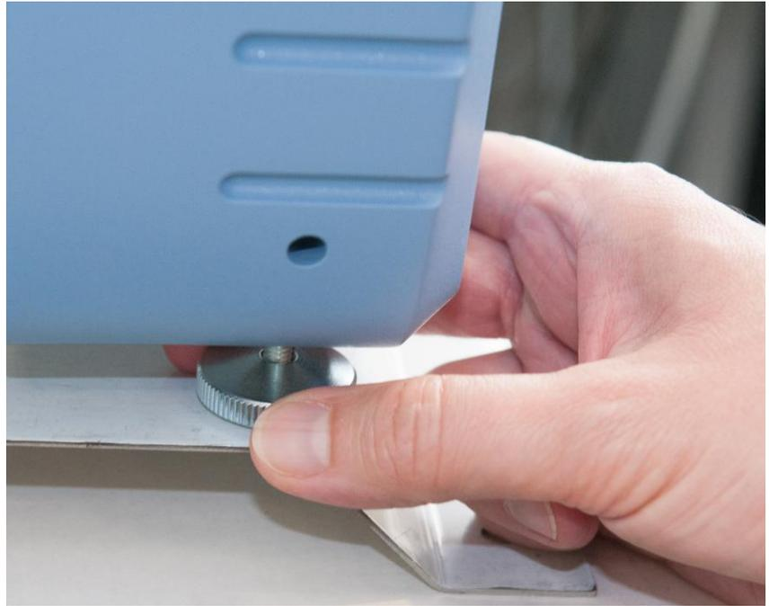
10. Now with the adaptor swung to the open position, insert the spray shield extender into position as shown and tighten the retaining screw.
