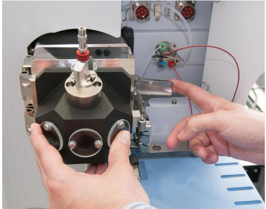
19. Reconnect the gas and liquid lines to the nebulizer.
