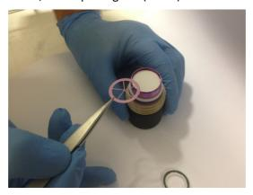
Then press the PTFE part assembled with o-ring firmly back in place
