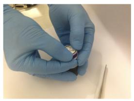
Finally, screw the filter block back into the ATLAS-SMA.
