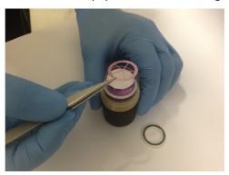
Remove the filter paper (50-0622) and discard this as appropriate for the chemicals which have been tested in the system.
