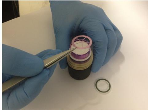
Remove the filter paper (50-0622) and discard this as appropriate for the chemicals which have been tested in the system.
