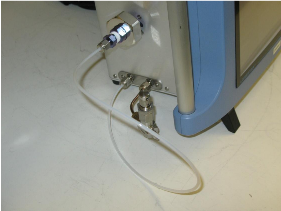
Figure 5 A photograph of a Lonestar unit set up within the Owlstone Quality Assurance department. Note the needle valve installed in the exhaust port and the loop of 1/8" PTFE pipe connecting the clean gas outlet with the filter mounted in the sample inlet. The filter tested within the Quality Assurance department is shipped with the Lonestar unit
