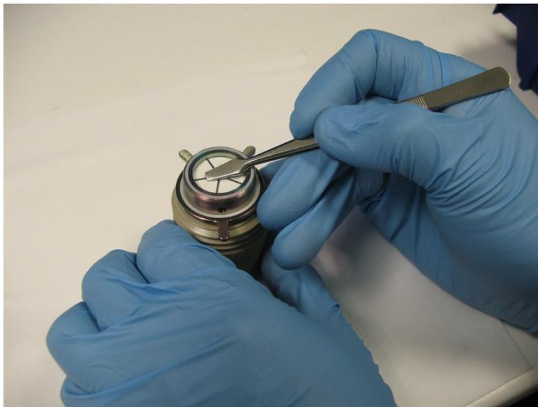
Figure 16 Removing the PTFE seal
