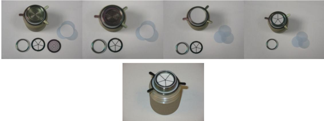
**Figure 17 Replacing the filter assembly**
