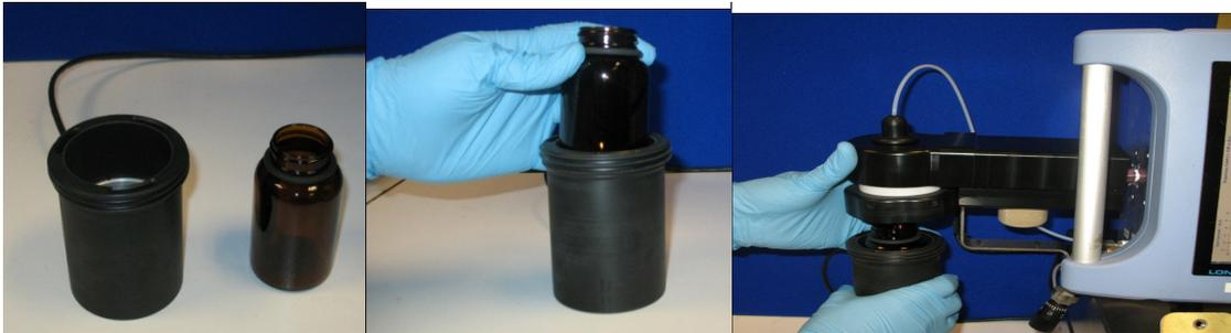
Figure 4 Mounting a sample
