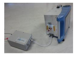
The pump inlet is connected to the Lonestar exhaust fitting, so the sample gas will be drawn through the Lonestar and subsequently through the pump.
