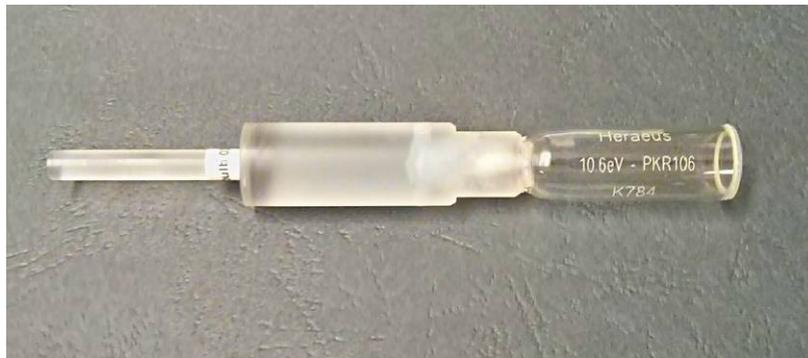
**Figure 9.** Bulb attached to holder.
