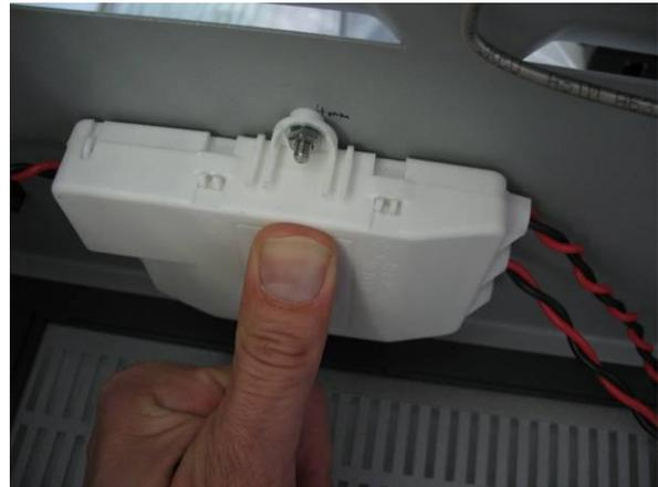
Figure 24 – closing the terminal box
