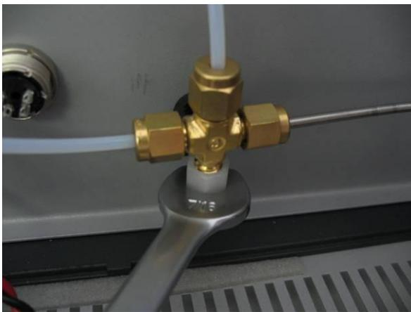
Figure 18 – removing the caps
