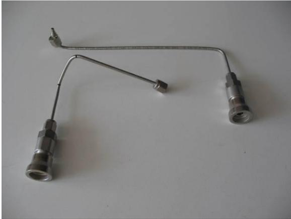
Figure 1 - Gas lines with quick connects
