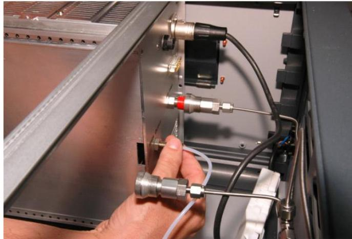
*Figure 11 – disconnecting the exhaust*
