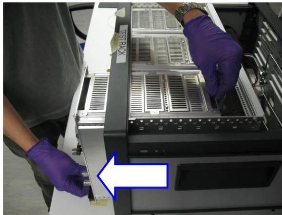
*Figure 12 – removing an OVG-4 from the GEN-SYS rack*
