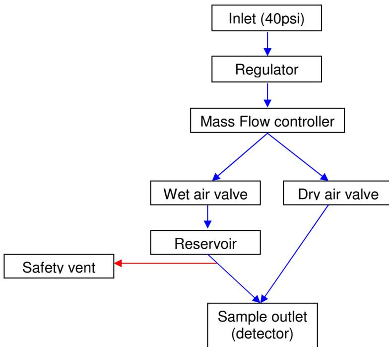
Figure 14 Schematic of flow path through the OHG-4
