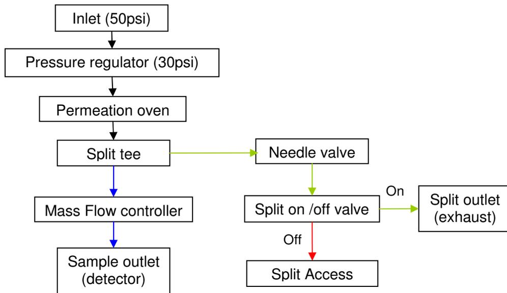
Figure 7 - Schematic of flow path through the OVG-4
