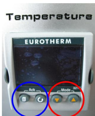
Figure 5 - Eurotherm temperature controller
