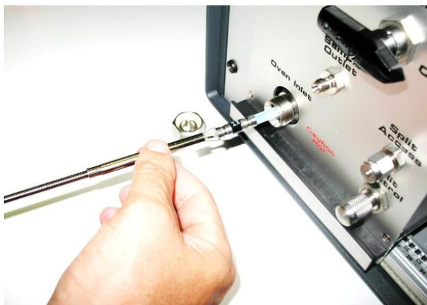
Figure 4 – Always use the supplied extraction tool
