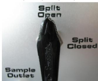
Figure 9 - How to change the split flow
