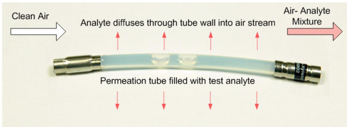
Figure 3 - Example of permeation device
