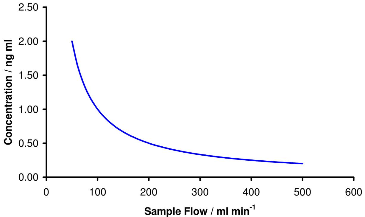
Figure 10 - Theoretical analyte concentrations at different sample flows, with an analyte permeation rate of  $100\text{ng min}^{-1}$  <sup>F</sup>
