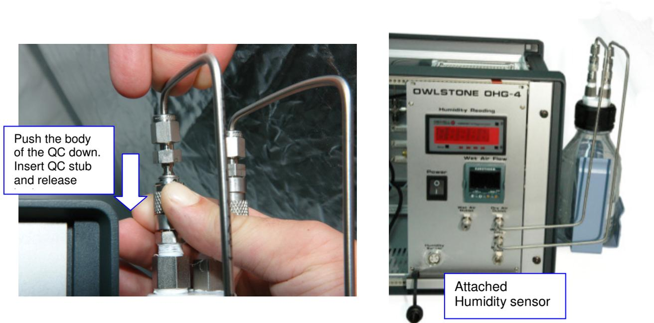
*Figure 33 - Connect water reservoir and the hygrometer to the OHG-4*
