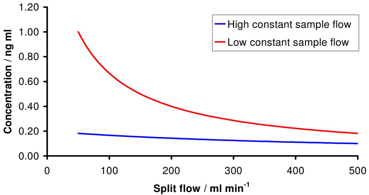
Figure 11 - Theoretical High and low constant sample flow concentrations at different split flows. Concentrations calculated using an analyte permeation rate of 100ng min<sup>-1</sup>
