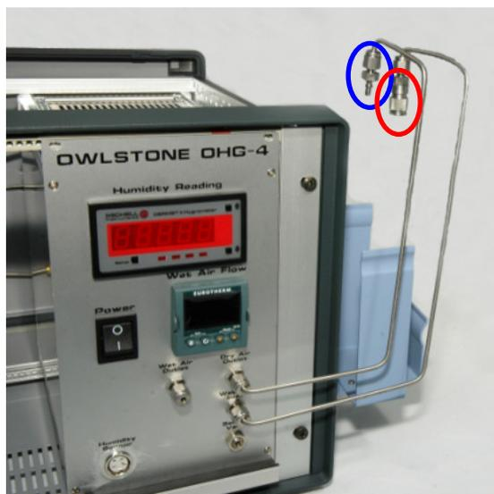
*Figure 32 Attach 1/8" tubing*
