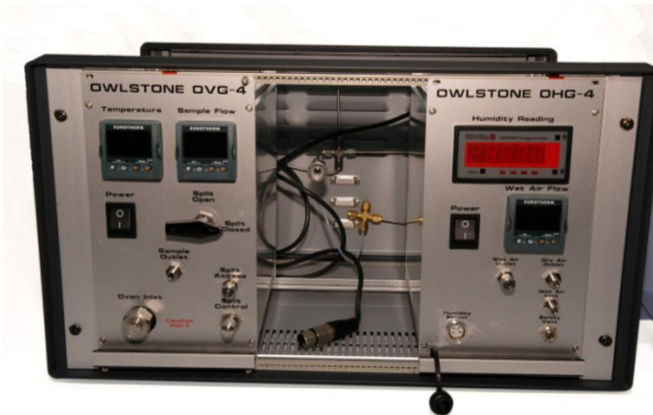
Figure 29 - Place OHG-4 in the GEN-SYS on the side with the reservoir holder
