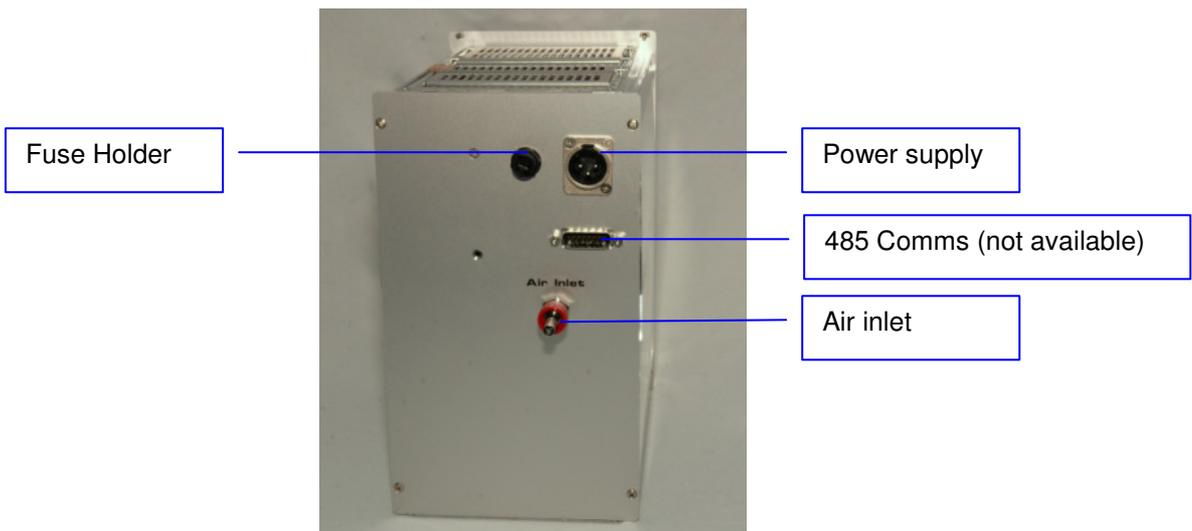
Figure 24 Back view of the OFC-1
