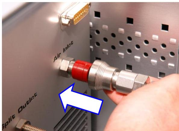
*Figure 20 - Connect Quick Connect Valve*
