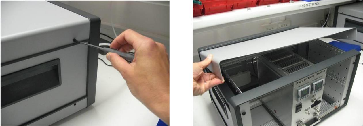
Figure 14 - removing the roof panel
