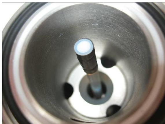
To insert a permeation source into the oven, first disconnect the air supply to the V-OVG and wait for the unit to depressurise. (Sample and Exhaust Flows should read  $0 \text{ ml min}^{-1}$ ). Unscrew the black lid of the oven, located on the top surface of the V-OVG.
