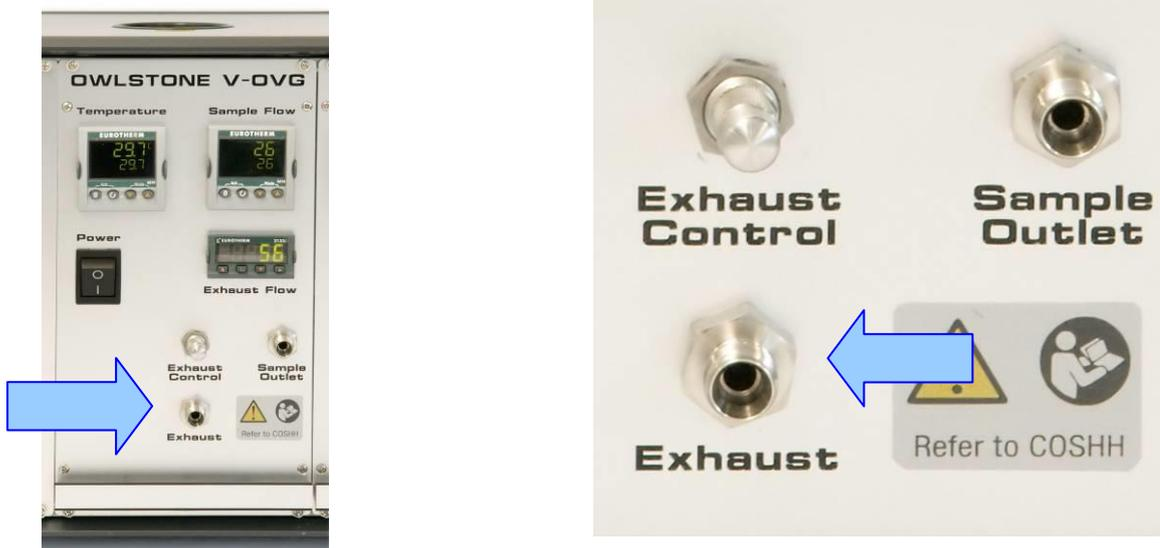
Remove the nylon cap from the Exhaust port on the front of each V-OVG sub-unit supplied with the system.
