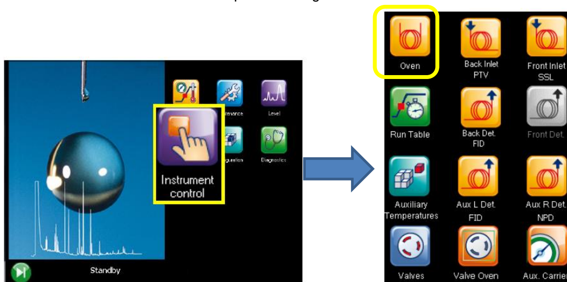
Figure 5. Instrument control menu. Press “oven” in order to enter the GC oven ramp rates configuration.
