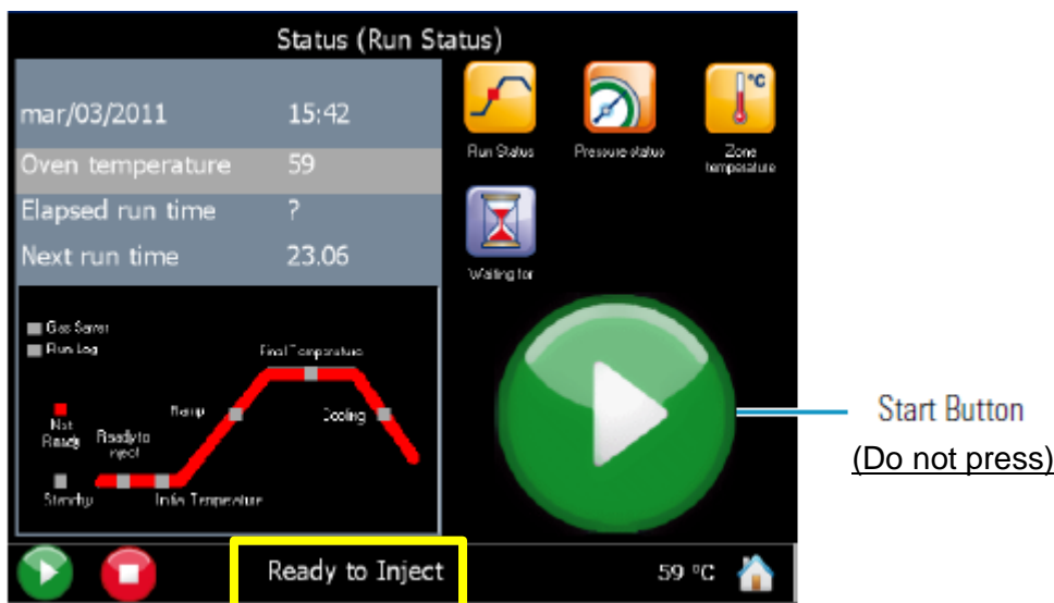
Figure 9. Ready to inject. Do not press the start button for sample analysis. Start button is only used for GC column blanks.
