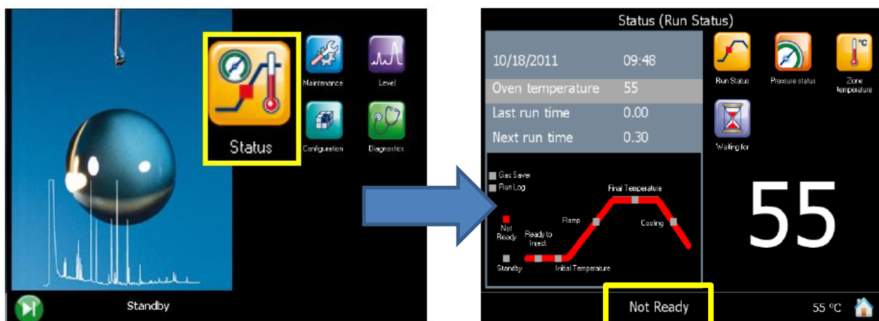
Figure 7. Status menu. Press on the “Oven temperature” to display the current temperature on the screen. In yellow, the current status of the GC. It requires to be “Ready to inject” in order to start the sample analysis.
