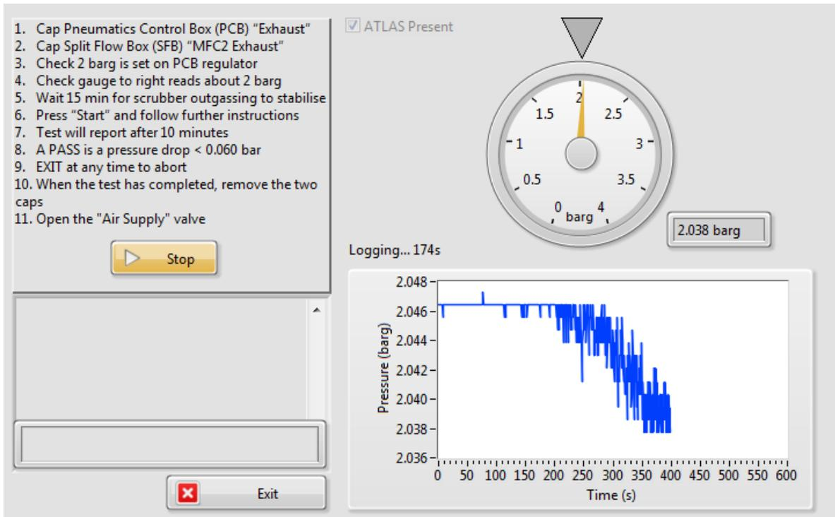
Figure 19. LNS pressure test in progress.
