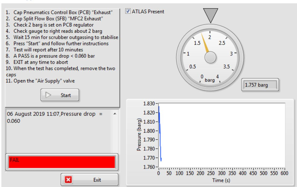
Figure 22. Example of Failed LNS Pressure Test. In this example, the blanking cap inspection showed the MFC1 out was not capped. The test passed after resolving it.
