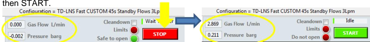
Figure 21. How to restore gas flow and pressure parameters on the LNS.
