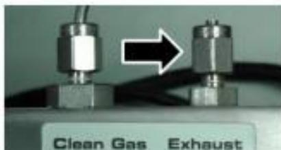
Figure 14. 1/8" Swagelok blanking nut capping the ATLAS pneumatic box exhaust.
