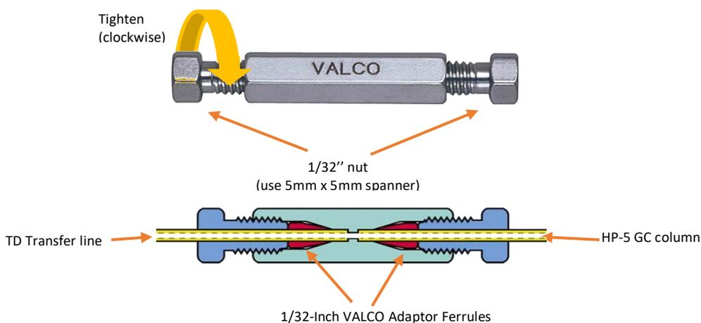
Figure 9. Diagram showing the different parts of the Siltek MXT connector kit. The 1/32" nuts are tightened clockwise and loosened anticlockwise.
