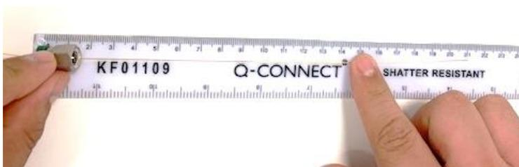
Figure 27. Measure 21cm from the cut end. Marks can be done with liquid typex or with a septum.
