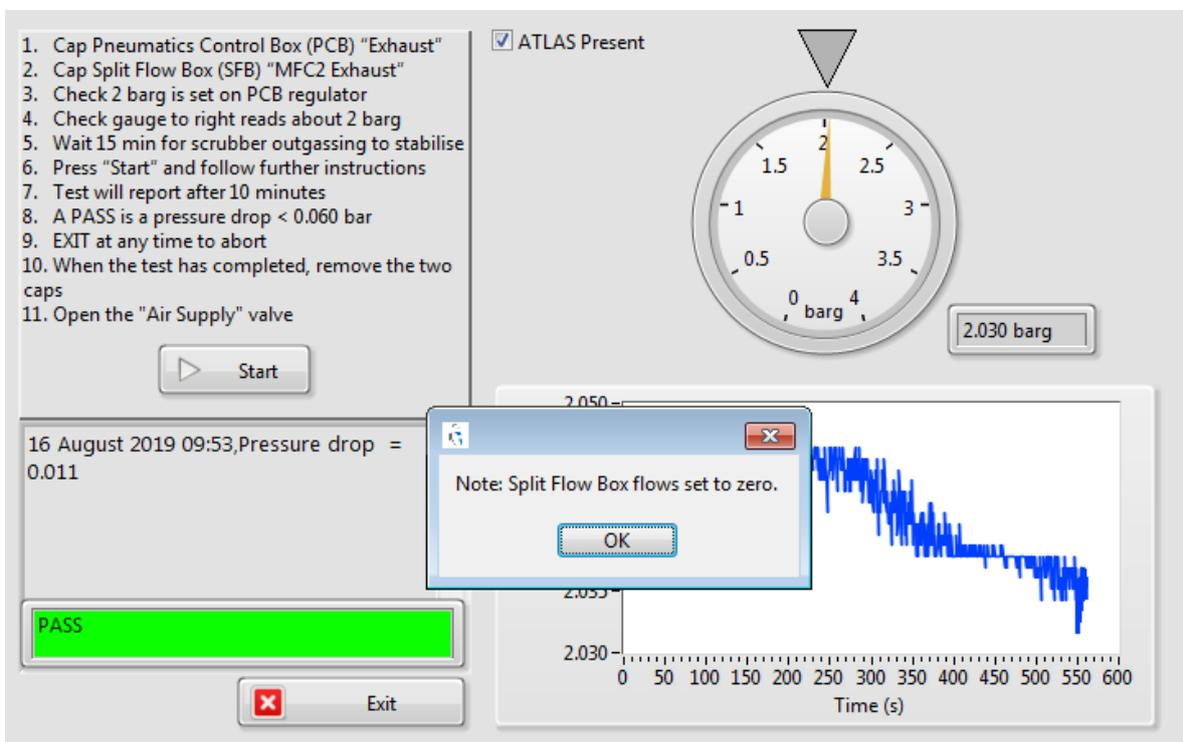
Figure 20. LNS Pressure test – Pass result screen.
