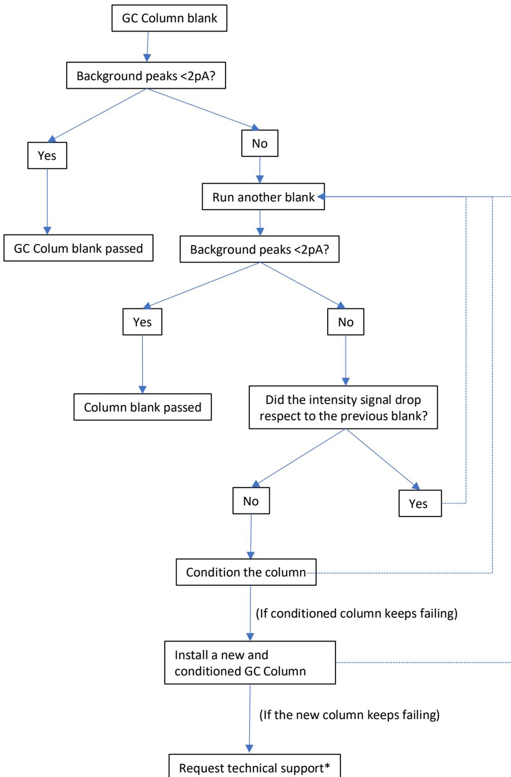
Figure 33. Steps in GC column blanking.
