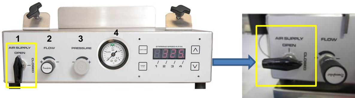
Figure 5. ATLAS pneumatic control box diagram. 1) Air supply valve, 2) Pressure Regulator, 4) Pressure dial.
