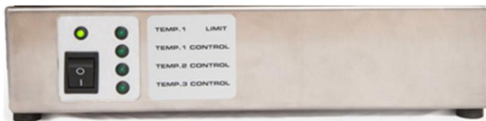
Figure 6. ATLAS heat box. The light panel displayed is how it should look like when the heat box is switched off.
