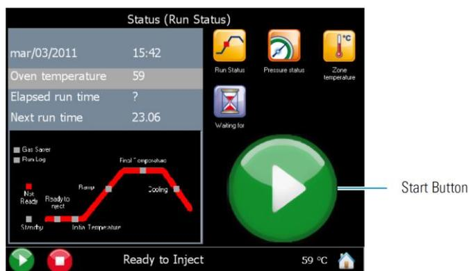
Figure 31. How to run a GC column blank: wait until the GC's status is “Ready to Inject” and then press the start button.
