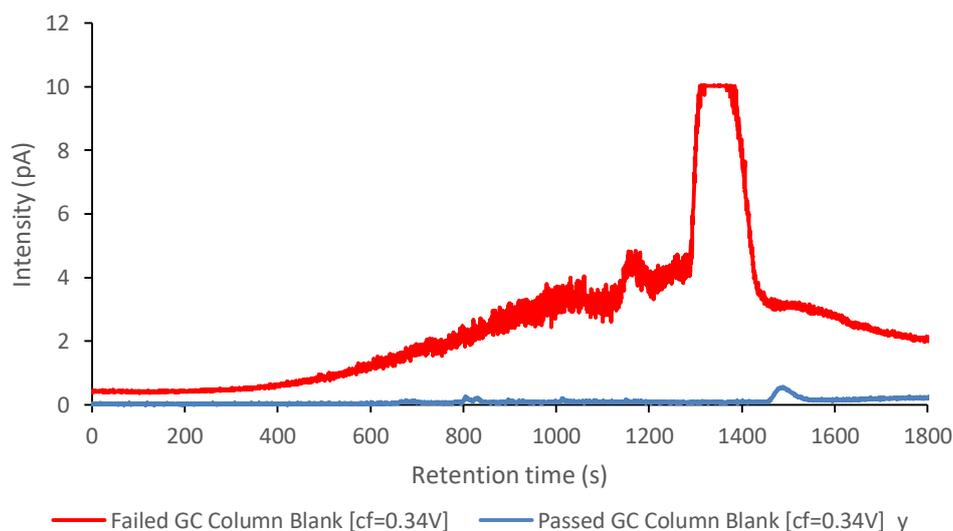
Figure 32. Comparison between and acceptable blank and a failed blank.
