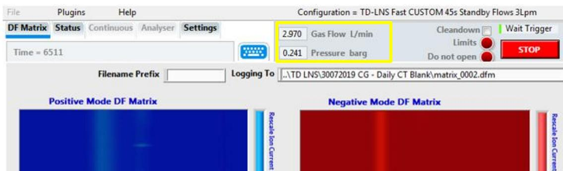
Figure 29. Location of the LNS gas flow and pressure parameters in the LNS interface.
