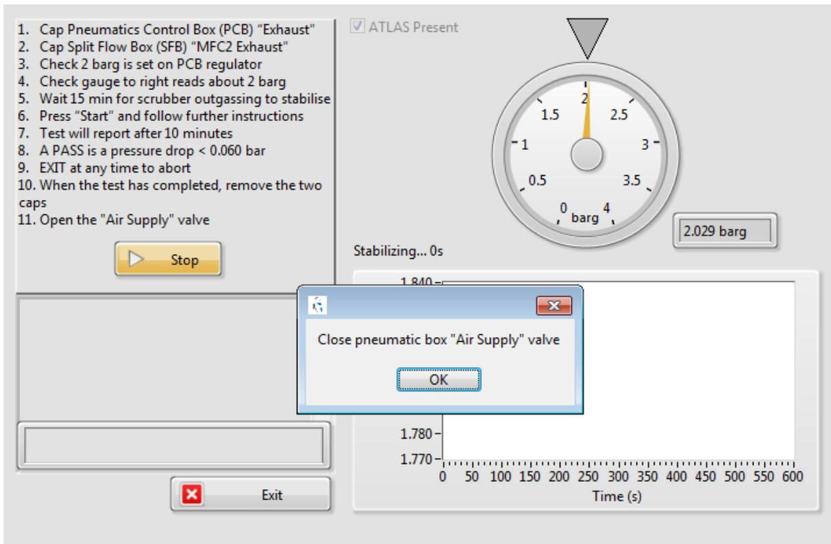
Figure 18. Close the pneumatic box after the pressure has stabilized. Once done, press "OK".
