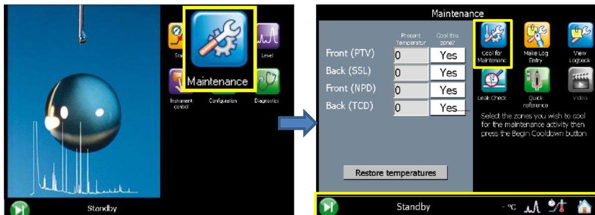
Figure 3. Cool for maintenance menu. The status of the system is displayed in the bottom bar of the interface.
