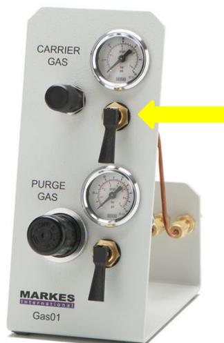
Figure 8. GAS01 secondary regulator. Use the carrier gas switch to close the line.
