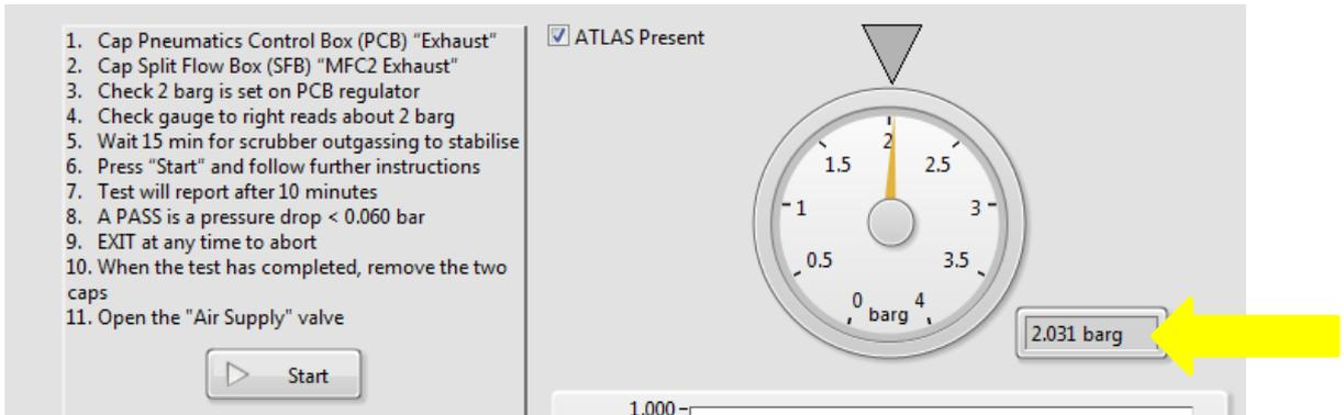
Figure 17. Check the gauge to the right reads about 2barg.
