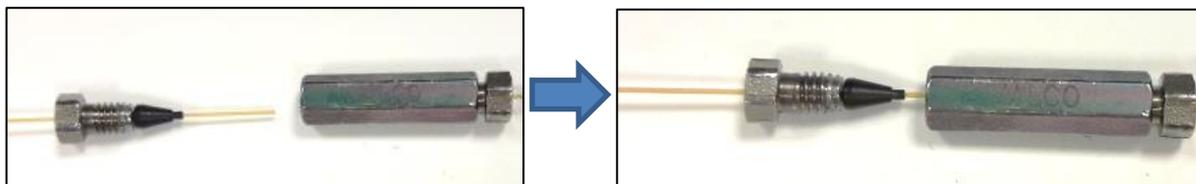
Figure 26. How to connect the GC Column to the Siltek MXT VALCO union. Leave a couple of cm from the GC column end and insert it into the union body. Pull then nut and finger tighten making sure the column end is fully inserted.
