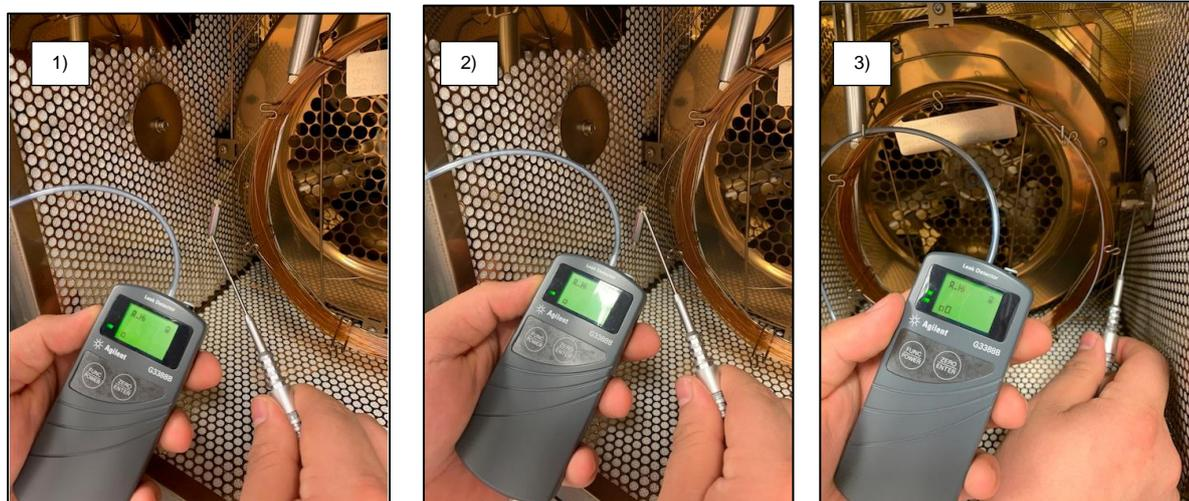
Figure 28. Pictures showing where to leak check. 1) Siltek MXT VALCO union, GC column side, 2) Siltek MXT VALCO union, TD transfer line side, 3) 1/8" Swagelok nut, connecting the GC column with the LNS transfer line. These connections must be tightened if the leak check fails.
