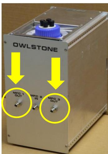
Figure 16. Split Flow Box front view. MFC1 out and MFC3 out required to be capped with a 1/8" blanking nut if they are not connected to the TD-GC-LNS system.
