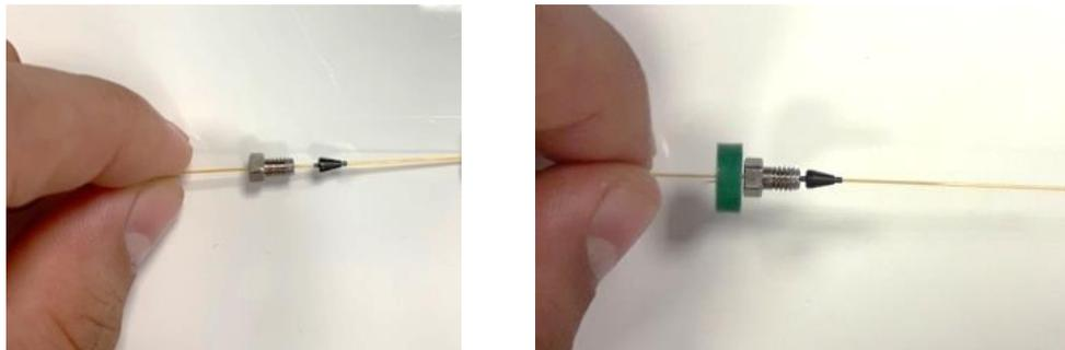
*Figure 23. How to insert the Siltek MXT VALCO union male nut and the 1/32" adaptor ferrules in a GC column. A thermostable GC septum can be used, but it is not essential.*
