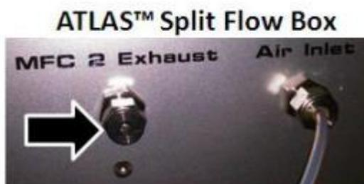
Figure 15. 1/8" Swagelok blanking nut capping the ATLAS Split Flow Box exhaust.
