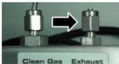
Figure 14. 1/8" Swagelok blanking nut capping the ATLAS pneumatic box exhaust.
