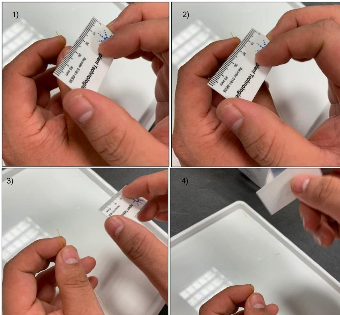
Figure 24. GC Column trimming technique. 1) Hold the end of the GC column. The cut is done in the GC section rest in the index finger. 2) Place the smooth side of the ceramic wafer perpendicularly to the capillary. 3) Gently, move the ceramic wafer alongside the finger to make a scratch on the capillary surface. 4) Flick the column to cut the column. If done properly, the cut should be straight and clean.
