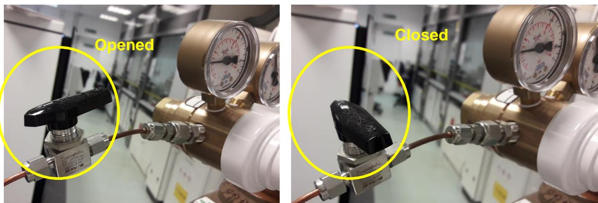
Figure 7. How to close the carrier gas line's toggle valve. From the “open” position (valve orientated parallelly to the gas line), turn it 90 degrees (valve orientated perpendicularly to the gas line) to close the carrier gas.
