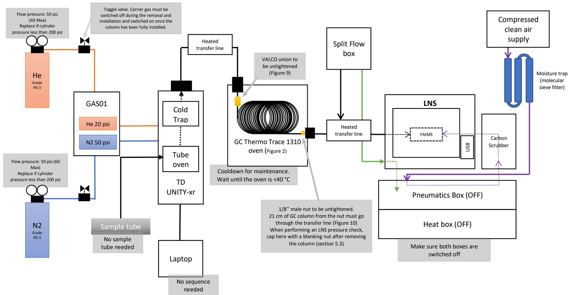
Figure 1. TD-GC-LNS diagram, with key steps to follow when removing a GC column.
