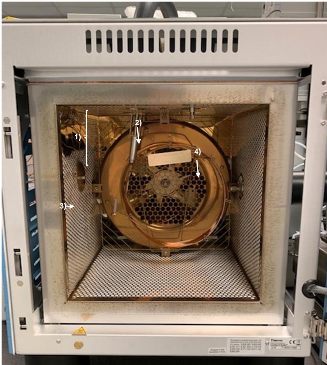
Figure 2. GC Thermo Trace 1310 oven. 1) TD Transfer line inlet, 2) HP-5 GC column held in the oven rack, 3) Siltek MXT VALCO union connecting the TD transfer line to the GC column (GC column end needs to be loosened), 4) GC column outlet. 21 cm of column goes through the 1/8" nut and connect with the LNS transfer line (needs to be loosen).
