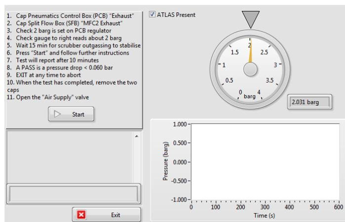
Figure 13. How to run a pressure test on the LNS system.
