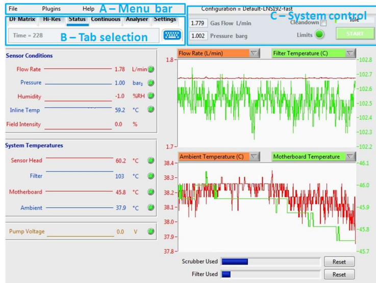
Figure 5: Status screen obtained from the Advanced button, showing the main Lonestar® software navigation bar and the three subsections.
