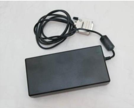
The power supply consists of a 24V power supply “brick” with a custom connector.
