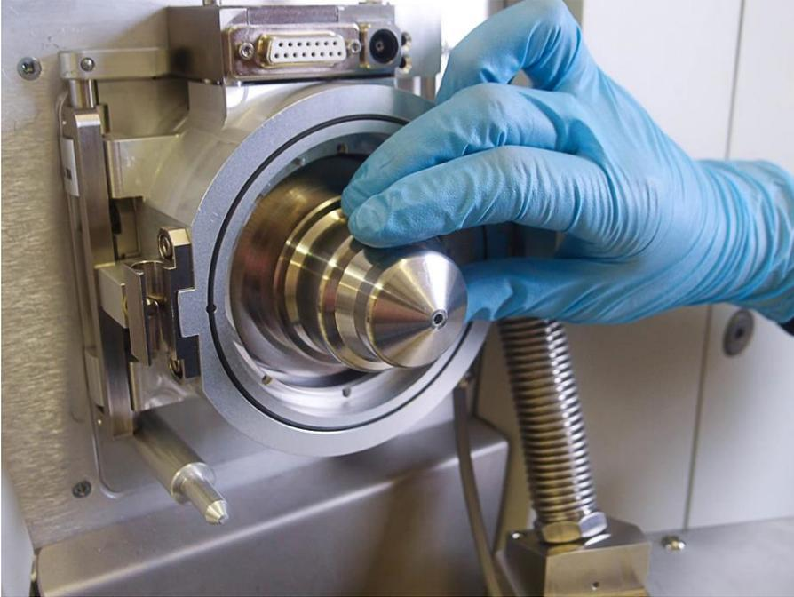
2. The PTFE **chip sealer assembly** is held in place in the cap by a single catch. To remove the **chip sealer assembly**, depress the catch (which can be accessed via the hole in the inner ring of the cap) using tweezers or other suitable tool, and lever the PTFE mount out. **IMPORTANT: do not try to remove by pulling on the gold connector pins as this may damage the chip.**
