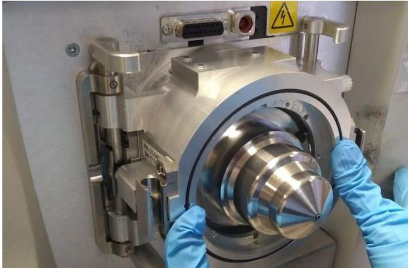
10. Rotate the rods to hold the **adaptor plate (ring)** in place.
