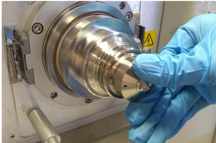
8. Screw in the chip cone (cap) outer part and tighten. **Tightening this sufficiently is essential** as this pushes the small o-ring inside the **T1 back cone** onto the capillary on the mass spectrometer to form a seal.
