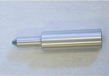
The support extender pin fits over one of the ionisation source support pins to allow the source to be supported when the adaptor plate is in place.
