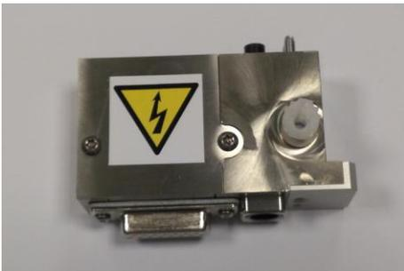
The connection extender is the interface between the mass spectrometer, and the ionisation source extending the gas and electrical connections to create the extra space needed for the FAIMS system to be fitted.
