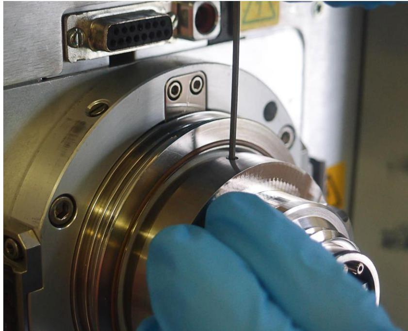
5. Choose the chip type to be used (NC or ND) and insert the chip sealer assembly into the **chip cone (cap)**, aligning the notch feature as shown
