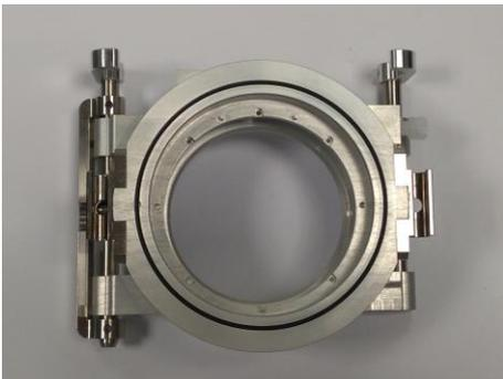
The adaptor plate (ring) is the interface between the mass spectrometer, the FAIMS module and the ionisation source.
