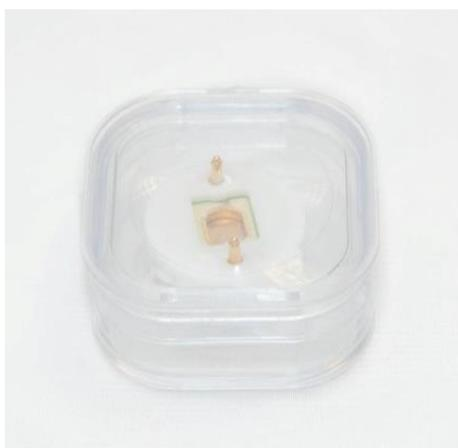
The chip sealer assembly (shown here inside the packaging) is the core of the ultraFAIMS system – this is the FAIMS device that produces the separation of ions as they pass through the fields applied across the channel.
