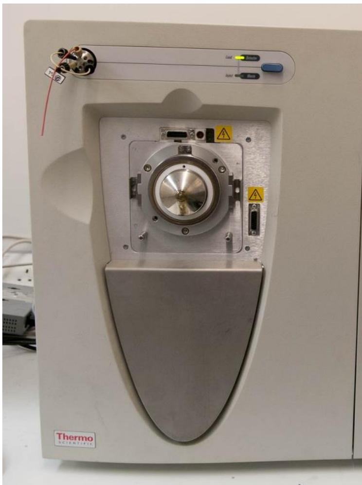
2. As supplied, the **chip cone (cap)** is screwed onto the **T1 back cone**. Unscrew this.
