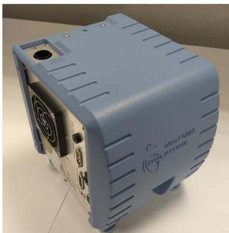
The control unit generates the FAIMS waveforms needed to drive the FAIMS chip.
