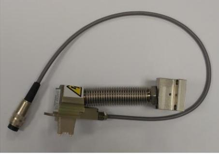
The RF waveform feeder connects the chip to the control unit so that the FAIMS waveforms can be applied. (Interlock sensor assembly is attached).
