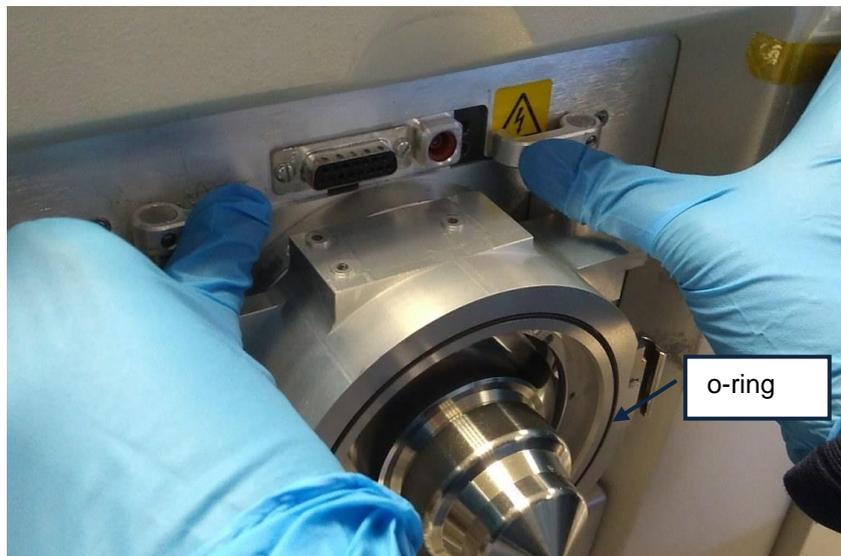
11. Fit the **connection extender** above the **adaptor plate (ring)**
