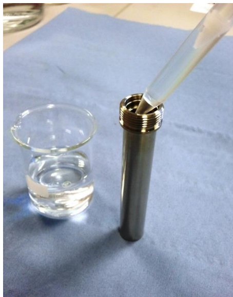
Figure 2 - Adding the chemical to the Wafer Device reservoir
