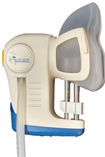
Switch on the CASPER. This gives the CO<sub>2</sub> sensor in ReCIVA time to equilibrate and flushes it with air ready to take a breath sample.
