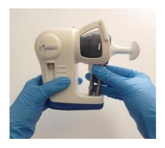
Push the Breath Biopsy Mouthpiece into the ReCIVA housing. Then, using fingers placed on either side of the white clamp, push the Breath Biopsy Cartridge firmly into the ReCIVA. Check to ensure both are fully seated into the ReCIVA.
