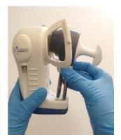
Now pull the Breath Biopsy Cartridge and Breath Biopsy Mouthpiece (with cartridge still inserted) forwards out of ReCIVA. They should come out easily.
