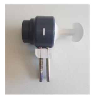
Insert the Breath Biopsy Mouthpiece and Breath Biopsy Cartridge loosely into the into the ReCIVA Breath Sampler.
